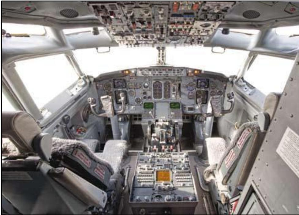
The Flight Deck has also undergone refurbishment which included repainting grey, new flooring, refurbished instrument panels, and refurbished flight deck seats which includes new foams and sheepskin seat covers.
